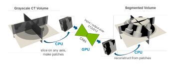
**CTSegNet** is a package for end-to-end 3D segmentation workflow for large X-ray tomographic datasets using 2D fully convolutional neural networks (fCNN).
